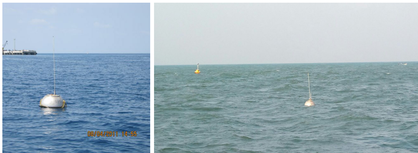
Figure 5: Datawell Wave Rider Buoy and the view of deployed buoys.
